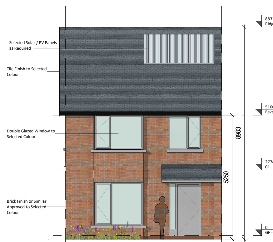
⑦ Front Elevation Type A (Full Brick) 1 : 100
